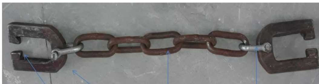
Fig A2 : Linking U-clamps
