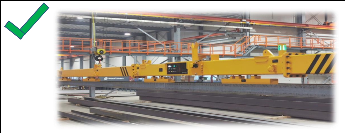
Figure 3.3 Magnetic Chucks for lifting steel
