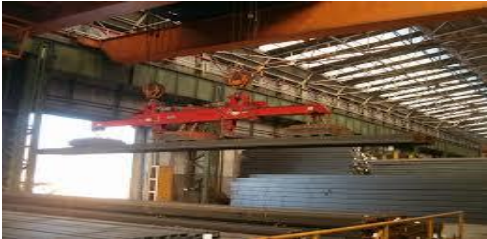
Figure 2.6: Electro-magnetic lifting device for lifting of rails in work shop.
