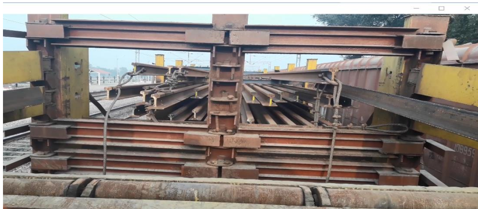
Fig 5.12: Two Layer Flap door opened for unloading Rail
