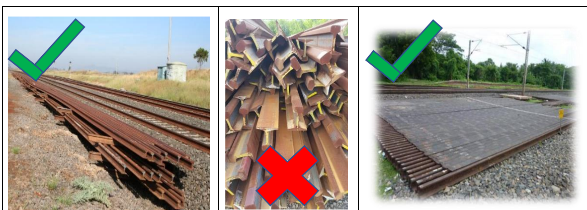
Fig 6.2 : Rails placed on cess in vertical position and supported @ 4m, spreader
