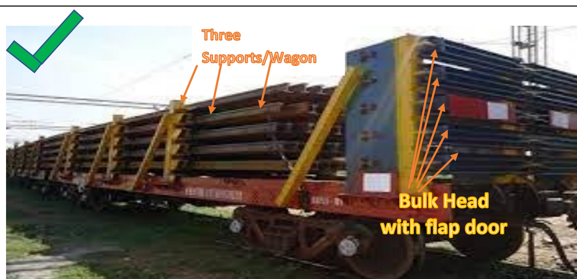
Fig 5.2: Three supports with rollers in between rails and Bulkhead with flap door
