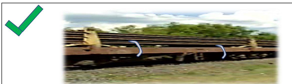
Fig 4.2: Loaded Rails tied together.
