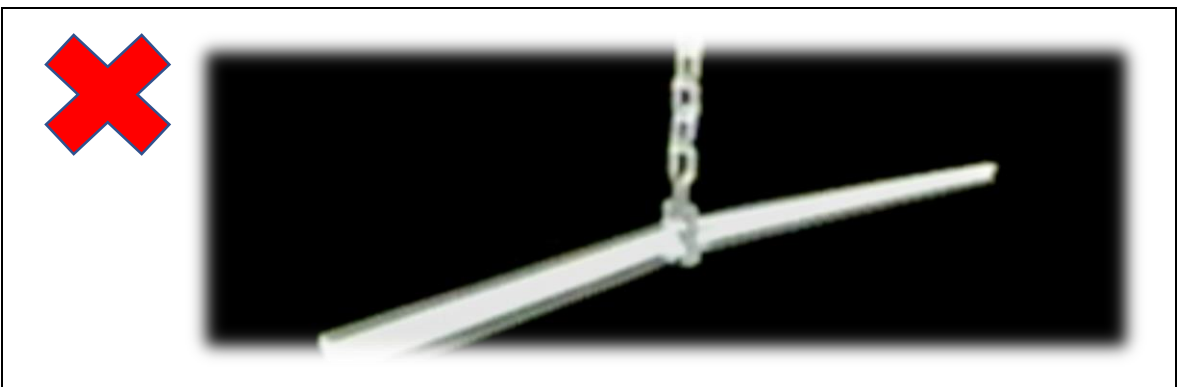
Fig 3.5 : Single point lifting of Rail
