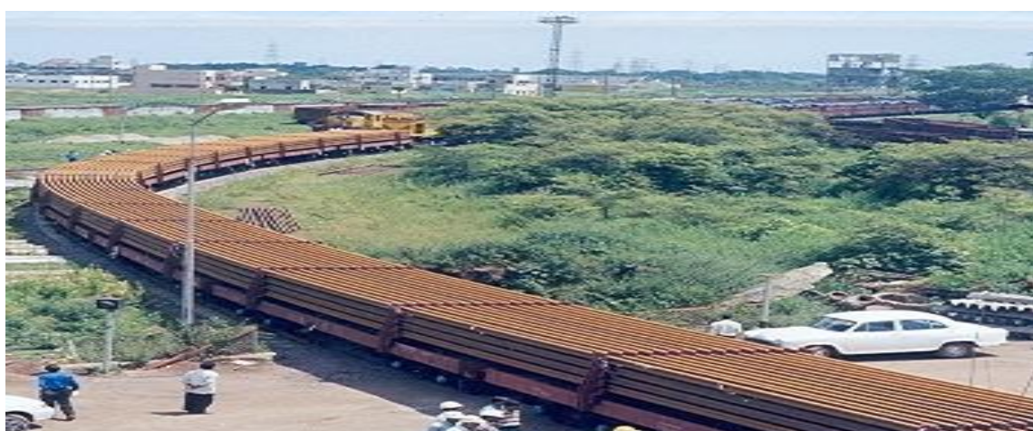
Fig 5.1: EUR rake with 20 Rail panel
