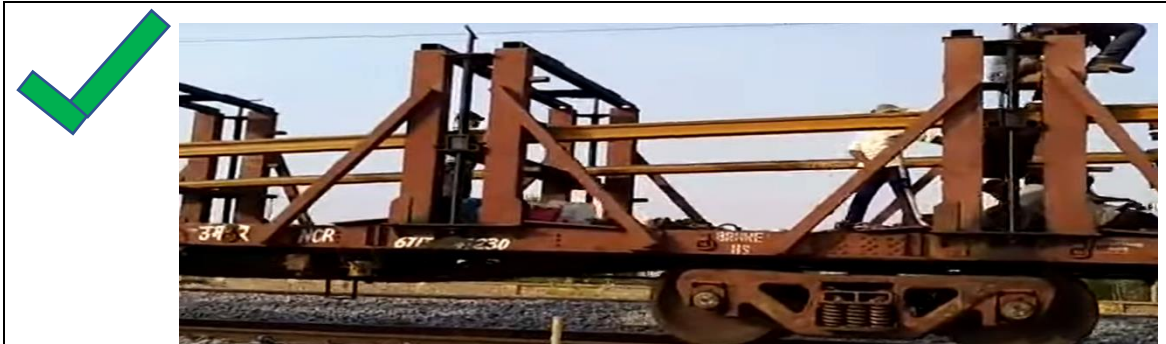
Figure 5.6: The adjustable ramp in threader wagon
