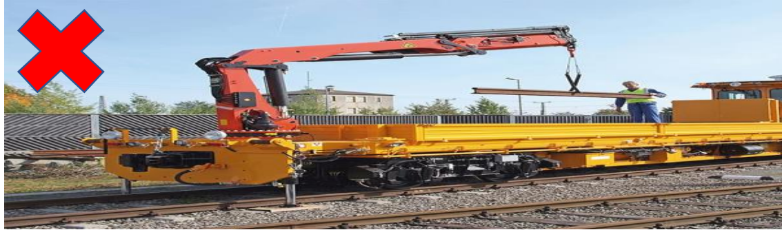
Fig 4.3: Unloading by UTV with lifting at centre
